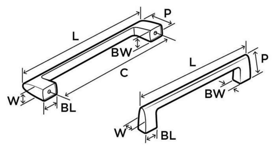
L (Length) = 8-15/16in(227mm) W (Width) = 1/2in(13mm)
